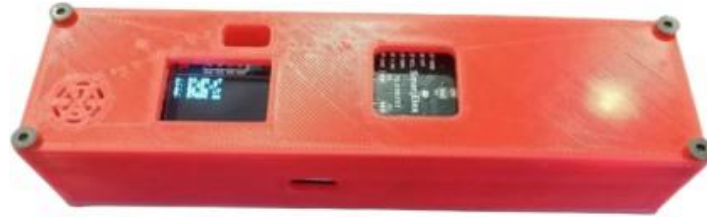
Figure 1: Assembled EMF monitoring prototype showing ESP32 module, MLX90393 sensor, OLED display, TP4056 power board, and 3D-printed PETG enclosure
